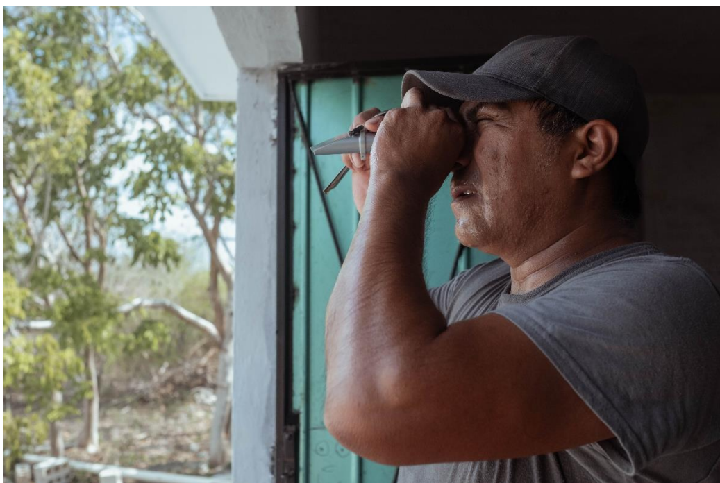
Diego Colli checks the density of water from a honey sample. Knowing how much water is in the honey helps the beekeepers to see how long it can stay fresh, the lower the water content the better the honey will keep.
